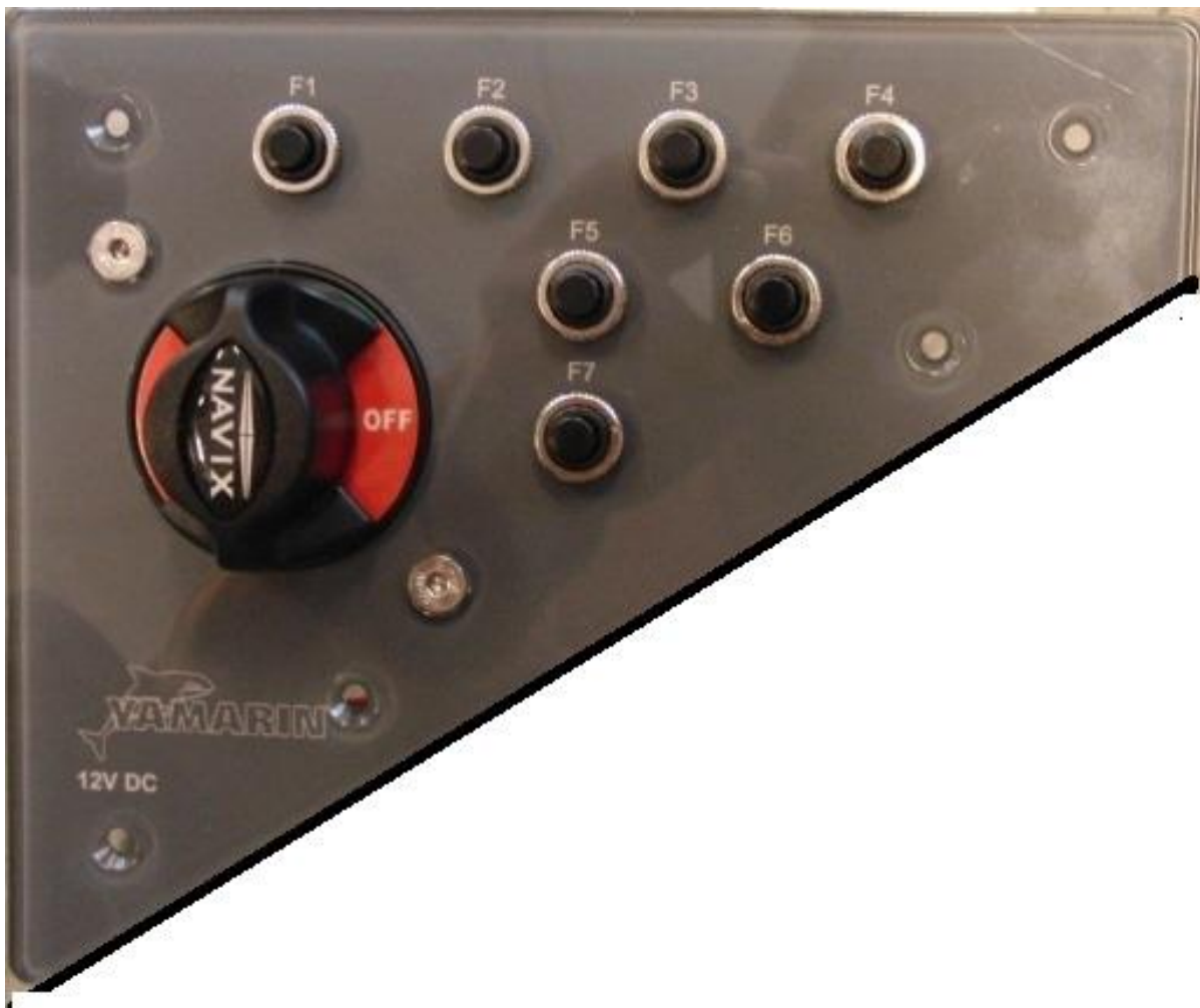
Image: Main power switch and circuit breakers.
