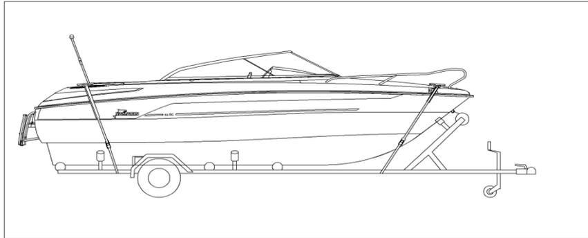
Tie the boat properly before starting the transport. Fastening belts located at the bow should be directed "down-back" and fastening belts located at rear should be directed "down-front". Do not leave any loose equipment or extra load to boat when it's transported. Take seat cushion away and close the hatches properly.
