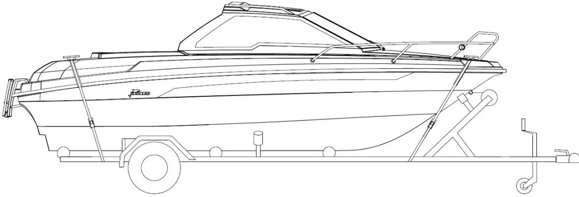
Image: Attaching the boat to the trailer.
