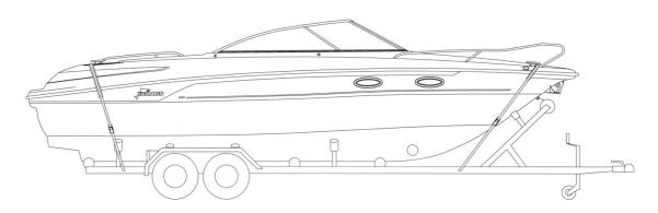
Image: Securing the boat to the trailer
