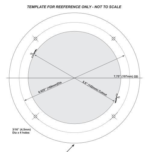
WATER DRAINAGE HOLE - DO NOT BLOCK
