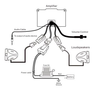
**Amplifier and Loudspeaker Mounting**
