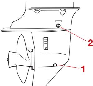
1. Gear oil drain screw
