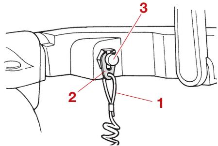
1. Engine shut-off cord (lanyard)
