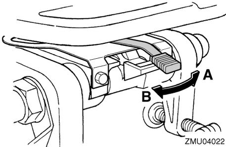
If the resistance does not increase even when the lever is turned to the port side "A", make sure that the nut is tightened to the specified torque.
