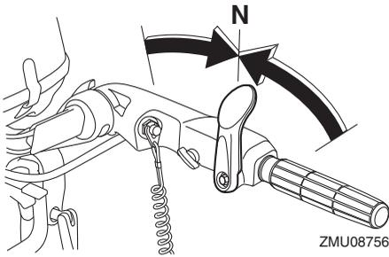
repeat the procedure. If the engine fails to start after 4 or 5 tries, open the throttle a small amount (between 1/8 and 1/4) and try again. Also if the engine is warm and fails to start, open the throttle a same amount and try to start the engine again. If the engine still fails to start, see page 46.
