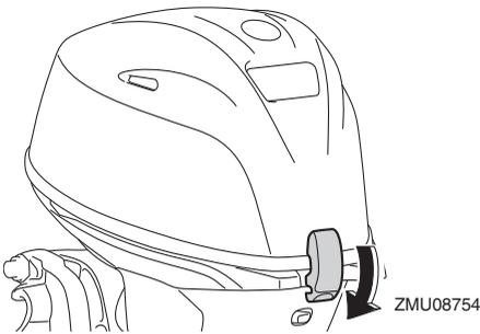
After installing, check the fitting of the top cowling by pushing it with both hands. If the top cowling is loose, have it repaired by your Yamaha dealer.
