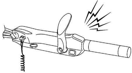
If the alert system has activated, stop the engine as soon as it is safe to do so. Check the oil level and add oil as needed. If the oil level is correct, consult your Yamaha dealer.
