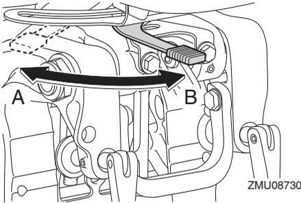
If the resistance does not increase even when the lever is turned to the starboard side “A”, make sure that the nut is tightened to the specified torque.
