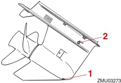
1. Gear oil drain screw
