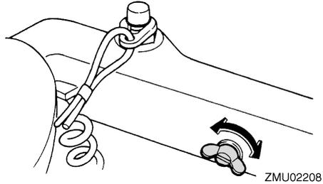
When constant speed is desired, tighten the adjuster to maintain the desired throttle setting.
