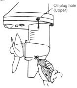
③ Install the upper oil plug, and then remove oil tube nozzle and install the lower oil plug.
