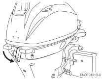
2. Remove starter lock cable from recoil starter by pulling the starter lock cable.
