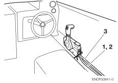
Install the remote control box in a position where it is easy to reach and operate the
