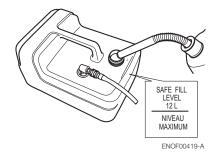
4. After filling the tank, close the fule tank cap.
