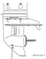
Insert the oil tube nozzle into the lower oil plug hole, and fill with gear oil by squeezing the oil tube until oil flows out of the upper plug hole and bubbles is disappeared to remove the air.
