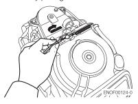
3. Remove the bolts (5pcs) and remove the recoil starter.
