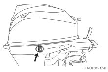
It is possible to tilt up or down in spite of main switch "ON" or "OFF".
