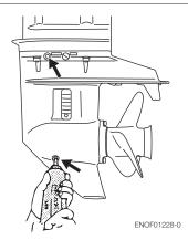
4. Install the upper oil plug, and then remove oil tube nozzle and install the lower oil plug.
