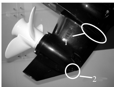
1. Oil level plug screw 2. Drain plug screw
