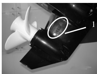
1. Cooling water inlet
