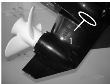
1. Oil level plug screw
