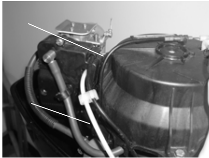
1. Start-in-gear protection device cable 2. Chock lever cable
