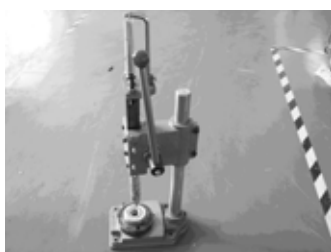
Oil seal installer tool
