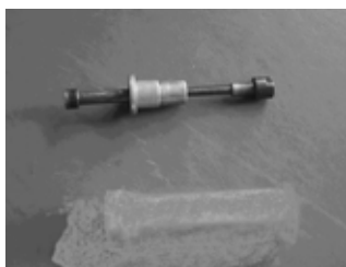
Barrel bearing with guard board installer tool
