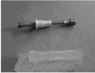
Barrel bearing with guard board installer tool
