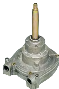
Y23 Helm (non self-centring fast-connect system)
