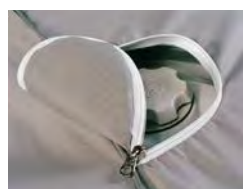
Fuel filler access
