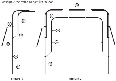
First assamble one side of the frame and slide the bimini top on the frame before assambeling the other half of the frame.
