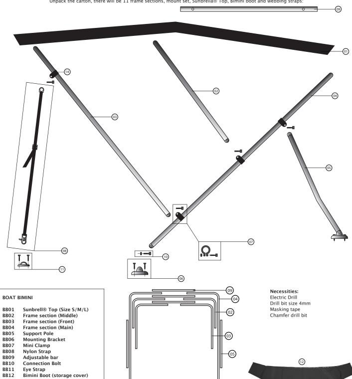
Prior to assembly, make sure all the required parts are present.
