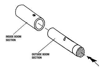
STEP 9: Take outside boom section with cables and slide into end of inside boom section until pin snaps into pin hole.
