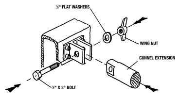
STEP 7: Take gunnel extension piece and place flat end with ½" hole into clamp. Put ½" x 3" bolt with ½" flat washers through clamp and gunnel extension and tighten wing nut to secure this piece. *Make sure wing nut is always secure during use*.
