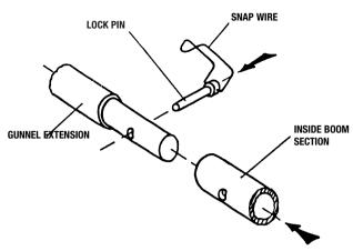
STEP 8: Take inside boom section and feed it through U boom stabilizer across boat until end of this section fits over end of gunnel extension piece. Place the lock pin through both holes in these sections. Be sure to snap wire over lock pin to assure it stays in position (adjust plastic gunnel protector so it rests properly on gunnel).
