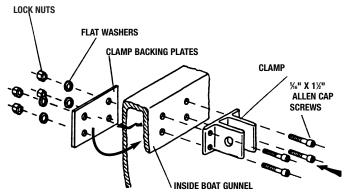
STEP 2: Take clamp and position it inside gunnel so the end of the boom will be about chest high for an average height skier. It is okay to angle the boom up to do this. Just make sure the gunnel is strong where you put the clamp.
