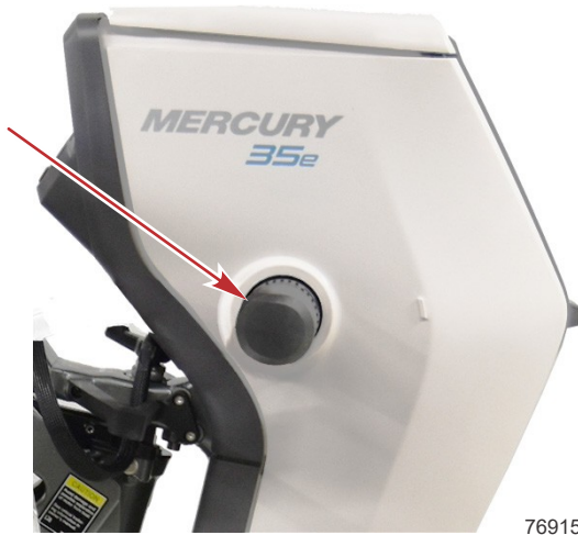
Weather cap installed
