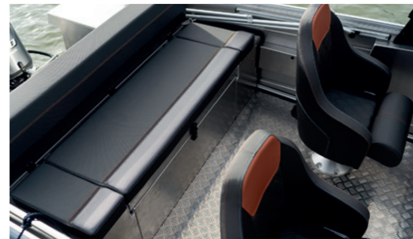
Aft seat with a lockable stowage, serves also as a fishing platform
