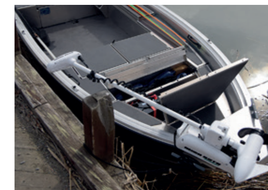
Casting deck for bow and motor bracket
