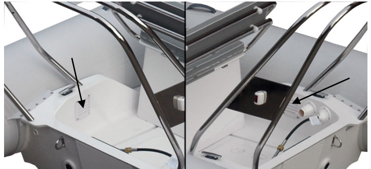
Fig. 2. Ventilation openings on the rear area.
