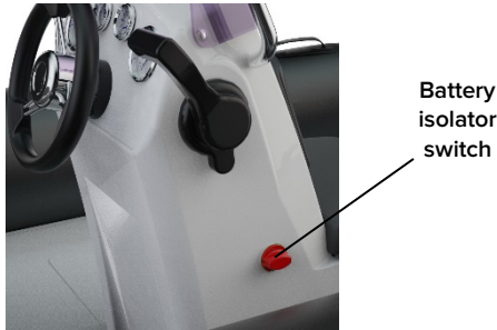
Fig. 22. Battery isolator switch.
