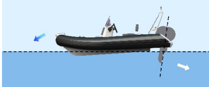
Fig.20. Trim down. If the motor is tilted too far inwards towards the transom the boat will travel bow down.
