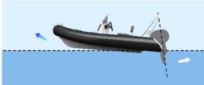
Fig. 19. Trim up. If the motor is tilted too far outwards from the transom, the boat will tend to porpoise.
