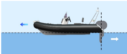
Fig. 18. Optimum trim. The optimum position is with the propeller axis parallel with the water.
