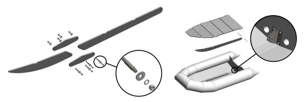
Fig.8. Assembly of wooden keel.
