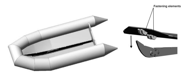
Fig. 10. View of installed keel.
