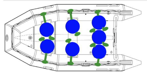
Fig.30. Recommended seating arrangement for 7 passengers.
