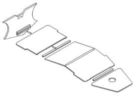
Fig. 5. How to assemble a floor. Step 1.
