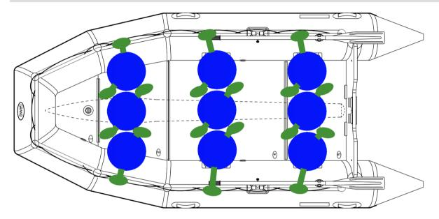
Fig.31. Recommended seating arrangement for 9 passengers.
