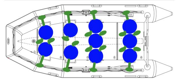
Fig.32. Recommended seating arrangement for 10 passengers.
