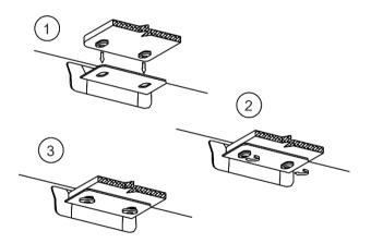
Fig. 17. Installation of wooden seats.
