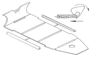
Fig. 7. How to assemble a floor. Step 3.
