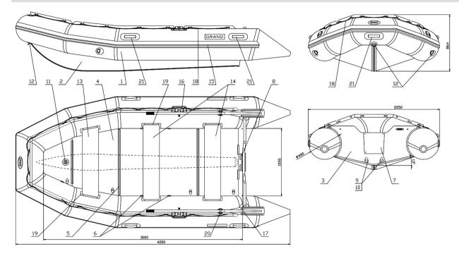
Fig. 27. General arrangement of a boat R420.
