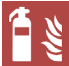
Fig.3. Symbol of designated place of portable fire extinguisher.
