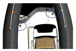
Fig. 28. Bow lifting eyes, 2 positions.
