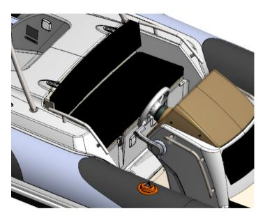
Fig. 31. Rear locker with access panel, lifters, soft seat and seat back.
