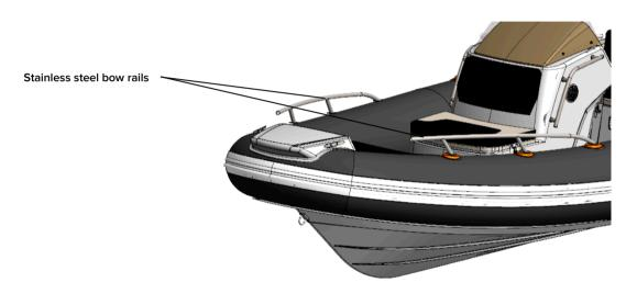
Fig. 33. Stainless steel bow rails.
