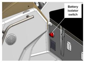
Fig. 19. Battery isolator switch.
