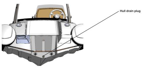
Fig. 26. The hull drain plug is located on the transom.
