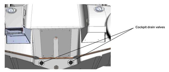
Fig. 27. Cockpit drain valves.
