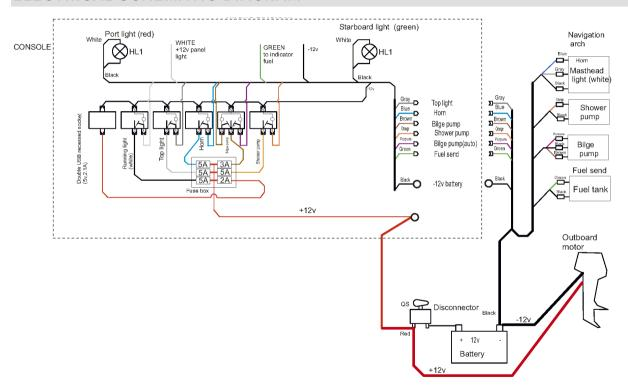
Fig. 49. Electrical schematic diagram.
