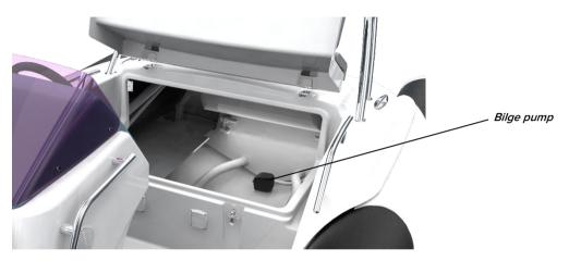
Fig. 23. Interior space of rear ccompartment with bilge pump inside of additional section.
