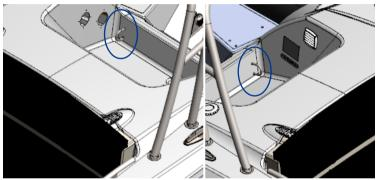
Fig. 29. Rear lifting eyes, 2 positions.
