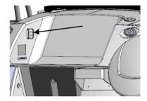
Fig. 3. Ventilation opening on the left side of transom area.
