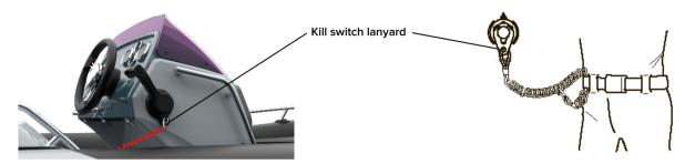
Fig. 18. Engine kill switch lanyard.
