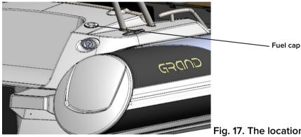
Fig. 17. The location of the fuel cap on the rear deck.
