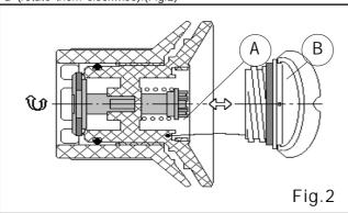
In order to discharge air from the compartments, open the valves (by counterclockwise rotation) and switch the valves over into condition "OPEN".
