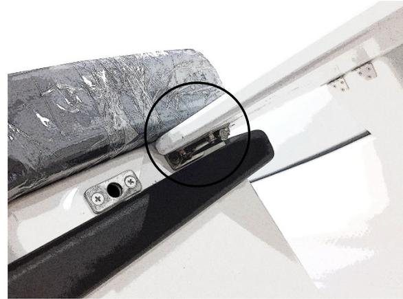
Install a pin into fixation hole.
