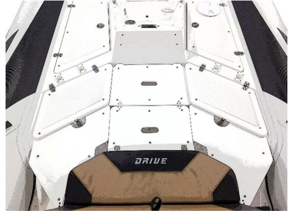
Fig. 49. How the rear sundeck should be installed.
