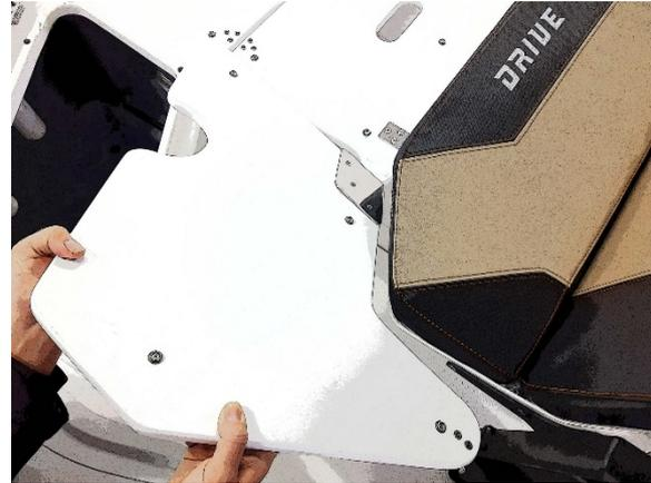
Fig. 48. How the rear sundeck should be installed.
