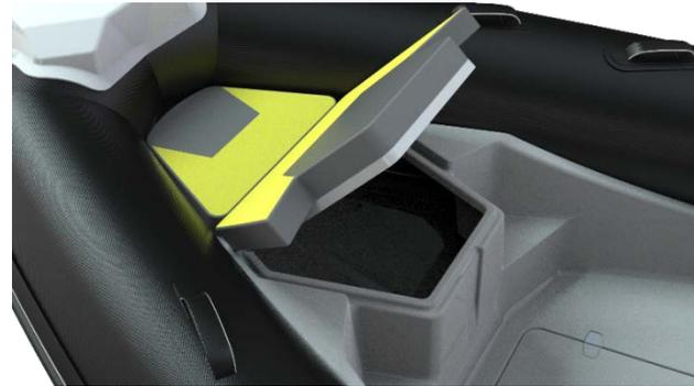
Fig. 34. Bow anchor storage and bow locker.
