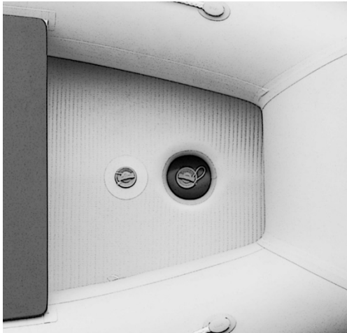
Fig. 8. Position of the inflatable floor against the keel valve.
